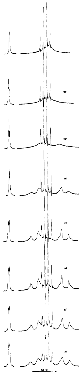
Figure 2. The methylene and vinyl regions of the pmr spectrum of Ia at temperatures above ambient. The solvent was toluene.
